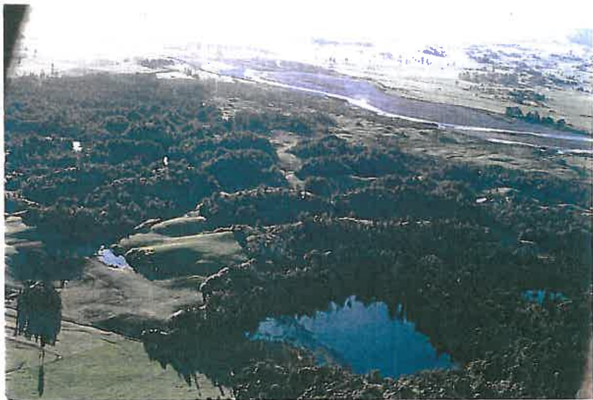
Figure 8.6 - The avalanche debris near the Kokatahi River forming Lake Arthur and adjacent lakes. The very smooth surface of the debris under pasture is a result of bulldozer regrading.
