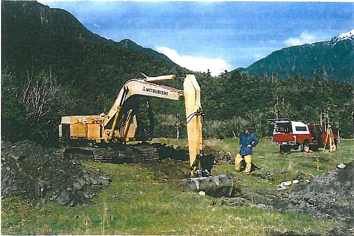
Figure 2.17 - The excavator at work beginning the Kokatahi 1 trench. The bucket is just starting to reach the actual fault rupture and blue grey coarse sand channel fill is visible immediately downhill of the bucket.
